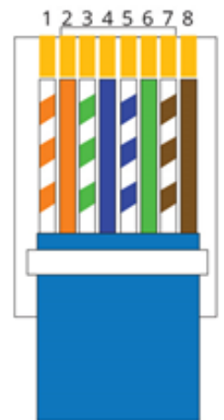
RJ45 Pinout T-568B
